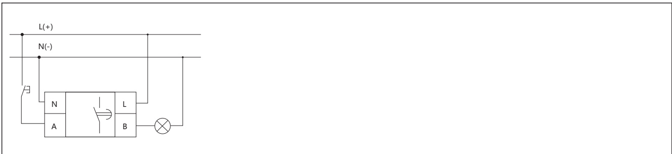
Figure 2 NTE8-□A Relay wiring diagram
