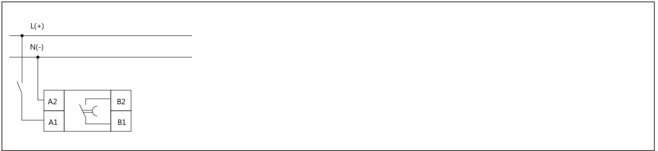
Figure 3 NTE8-□B Relay wiring diagram
