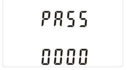
Setting up is password-protected so you must enter the correct password (default '1000') before processing. If an incorrect password is entered, the display will show: Err
